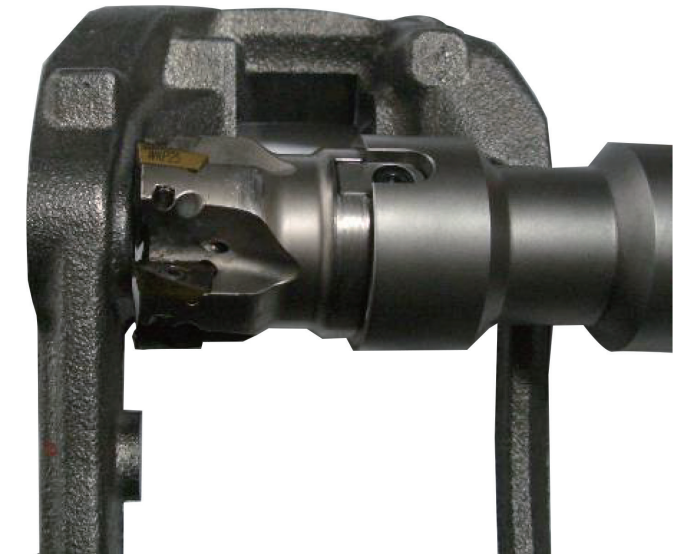
Application: Side milling Solution: Achteck AP series
