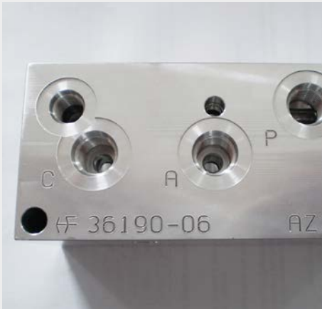
Marking of outer surfaces on a turning machine using needle embossing.
