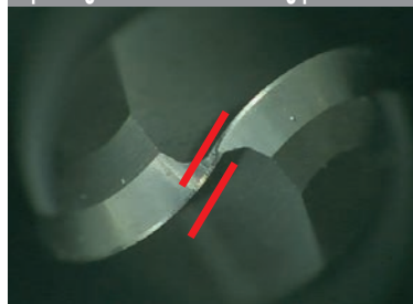
Tip design with excellent cutting performance
