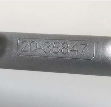
Marking of text, logos, etc. on flat or unfinished surfaces using needle embossing.
